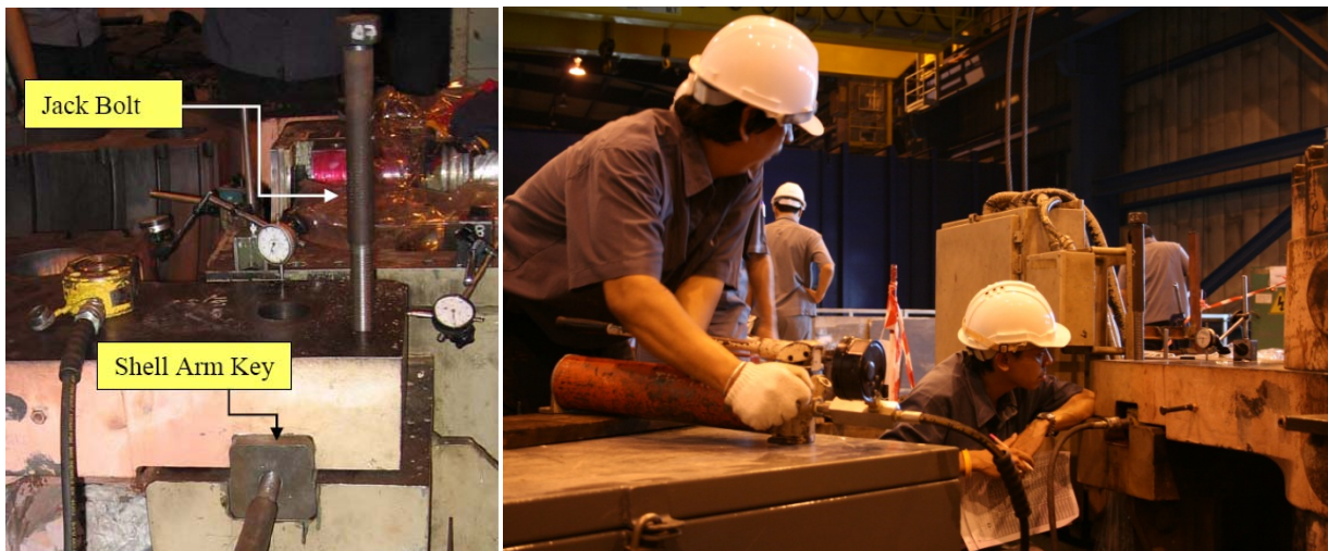
Figure 6 Hydraulic lifting the Front casing in the process of Horn drop test
