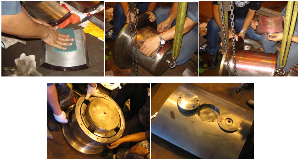
Figure 9 Bearing Inspection and Setting
