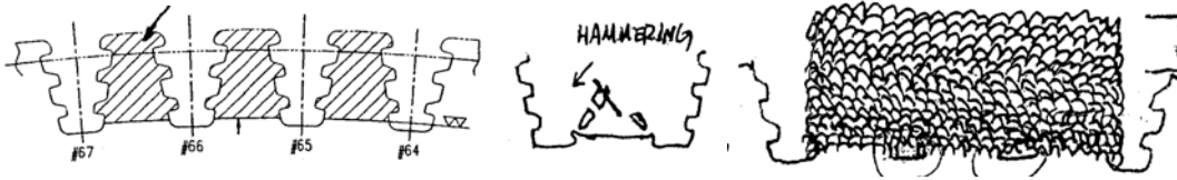
Figure 11 Schematic of welding repair steps
