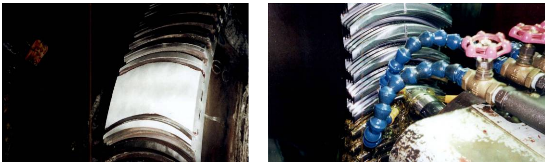
Figure 12 building up metal and re-machining on L-0 grooves (SB-T5)
