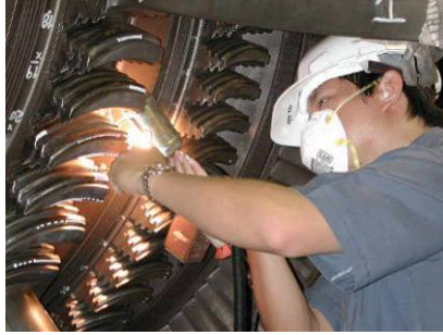
Figure 2 Replication test after several indications on rotor grooves were found
